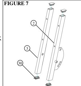
**STEP 9:**Insert four 2 X 1" END CAPS (30) into the ends of the BACK PAD ADJUST TUBE (2) & BACK PAD SUPPORT TUBE (3). See FIGURE 7.
